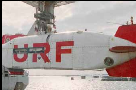
5. URF Submarine: Underwater vehicle for submarine rescue opera- tions. 35 persons at a time can be transported from a depth of 460 meters. Engine room protected by FS49C2
